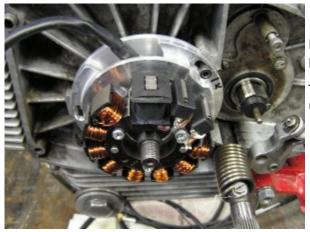
Place the new stator unit onto the engine, same place as the old stator plate had been sitting.
