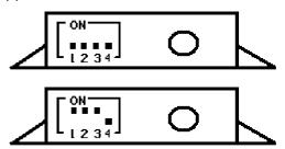
With all switches on OFF (opposite ON) the engine will reach full advance of 38° at 3.000rpm, as it should be.
