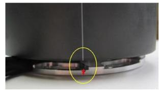
Place the rotor loosely onto the crank and check that it may move freely above the statorbase, check carefully that it clears the heads of the screws holding the inner plate to the adapter. Take the spark plug out and bring the piston into "TDC" (top dead centre) position. As this is difficult to do with the kick lever, using the rotor as a turning knob.
