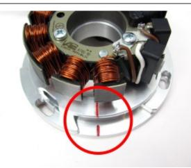
Have a look at the new stator unit. You will find there a near the smallerer black coils a small red marking. This is an ignition marking for timing.
