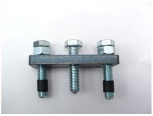
To disengage the new rotor use only the provided puller (part-no.: 76 93 799 34)!
