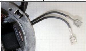
The 2 black wires running from the stator coil carry the voltage for lights, horn, flashers etc. They have nothing to do with ignition.
