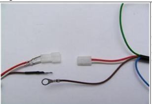
Look for the advance unit with its female plug and the two wires (red and white).
